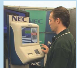
A wall-mounted unit with an access control terminal/seating monitor using fingerprint authentication technology in Chile.
